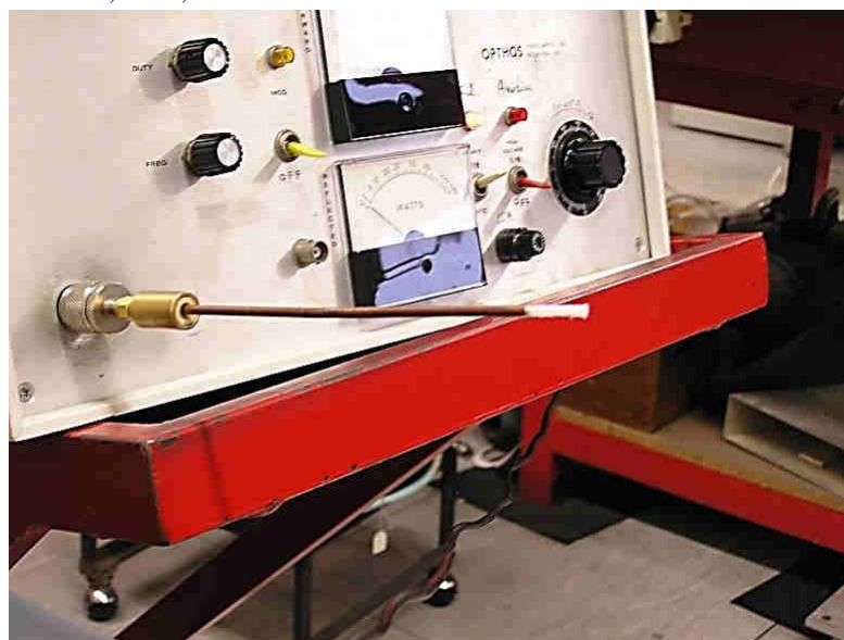
Fig. 2: Coaxial dipole antenna attached to the output port of microwave source. The dielectric-tip end is evident in the foreground.
